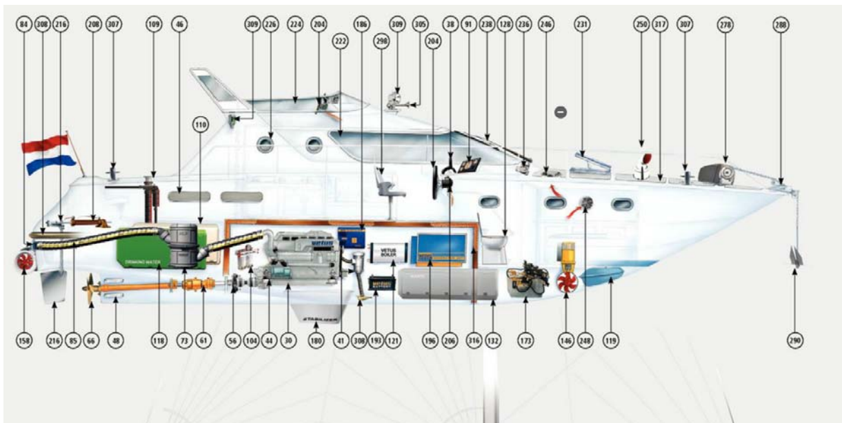
Figuur 1: The main components of a yacht. (taken from www.vetus.com (accessed 15-03-2013))
